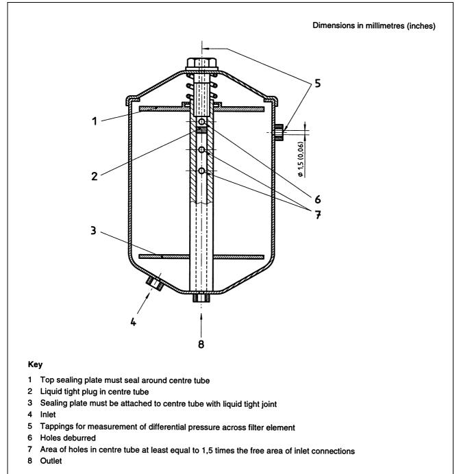
Figure 3 — Typical test housing
